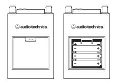
Battery Selection Each ATW-R1820 dual-channel receiver uses six 1.5V AA batteries, not included. Alkaline type is recommended. Always replace all batteries. Make certain the receiver power is Off before replacing batteries. Note: The ATW-R1820 receiver also functions without batteries if connected to an external power supply (12V DC source, 500 mA nominal current, not included).
